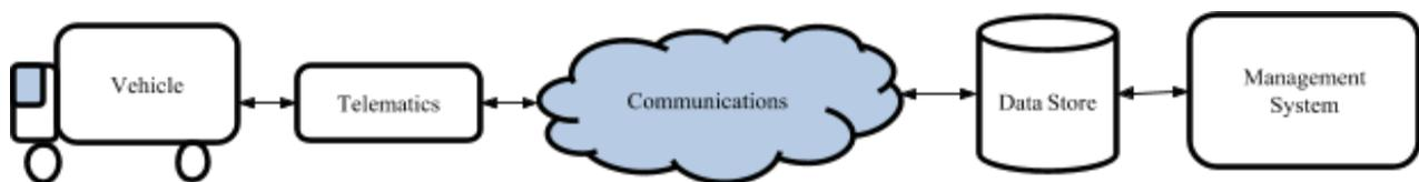
**Figure 1. Components of a Fleet Management Information System (FMIS)**
